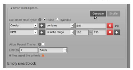
By default, a smart block will not contain repeated items, which will limit the duration of the block if you do not have sufficient items meeting the specified criteria in your **Library**. To override the default behaviour, check the **Allow Repeat Tracks** box.
