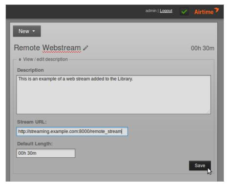
The **Stream URL** setting must include the *port number* (such as 8000) and *mount point* (such as remote\_stream) of the remote stream, in addition to the streaming server name. A **Default Length** for the remote stream can also be set. If the stream is added at the end of a show which becomes overbooked as a result, it will be faded out when the show ends.
