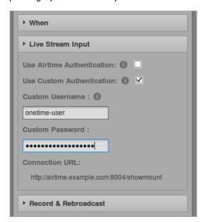
A reminder of the Connection URL for the live input stream to use is shown at the end of the Live Stream Input section.
