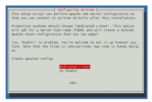
If so, you will need to enter the domain name that your station staff will use to access Airtime. For a test server that will only be accessed directly from the same machine, you can use the default setting of *localhost* here.
