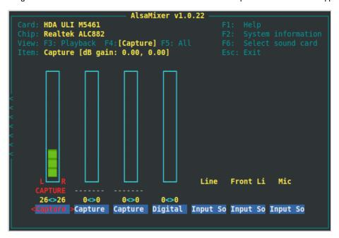
Press the **F4** key on your keyboard to set capture levels. Some experimentation may be required to find the correct control on the mixer, using the **Left** and **Right** arrow keys on your keyboard. Levels are set with the **Up** and **Down** arrows, and *Capture* is toggled with the **Space** bar. *Capture dB gain* should be set to 0.00, 0.00 initially.
