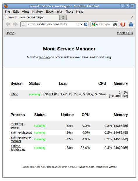
Clicking on the name of a service in the Process column, such as airtime-playout, opens another page with details of that service.
