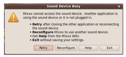
The solution is to configure Mixxx to use additional sound cards by clicking  $\mathbf{Options}$ ,  $\mathbf{Preferences}$ , then  $\mathbf{Sound}$   $\mathbf{Hardware}$  in the main Mixxx menu. Select devices other than the ALSA default of hw:0,0 for at least the  $\mathbf{Master}$  and  $\mathbf{Headphones}$  outputs. Then click the  $\mathbf{OK}$  button.
