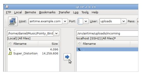
For additional security, you could configure your Airtime server to use an encryption key pair for the uploads account, instead of a password. See https://help.ubuntu.com/community/SSH/OpenSSH/Keys for details of how to do this on an Ubuntu server.
