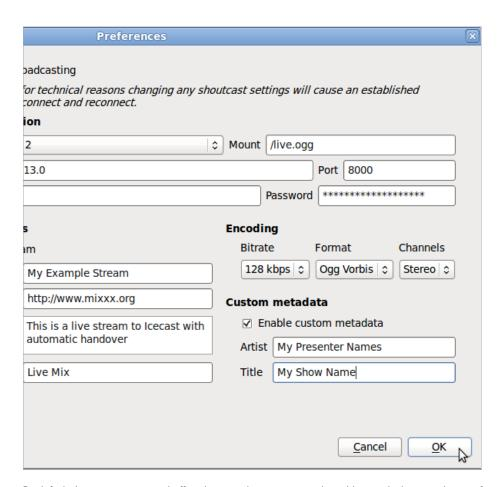
By default, Icecast streams are buffered to guard against network problems, which causes latency for remote listeners. When monitoring the stream from a remote location, you may have to begin the live stream a few seconds before the previous stream ends to enable a smooth transition.
